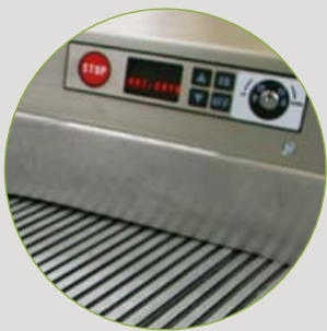
Emergency stop buttons
