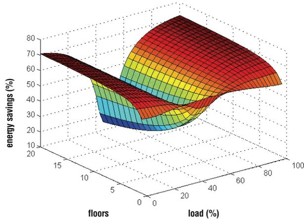
Energy savings with a ReGen drive versus a non-regenerative drive during elevator motion as a function of car load and elevator run from 1 to 20 floors for a typical elevator cycle
