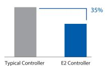
SNAP control increases passenger comfort by reducing low frequency car bounce up to 35 percent at the start and the end of the elevator run.
