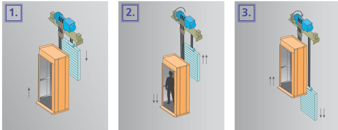
1. An elevator consists of a car and a counterweight that are connected by a machine. When the counterweight travels down, the car travels up and when the counterweight travels up, the car travels down.
