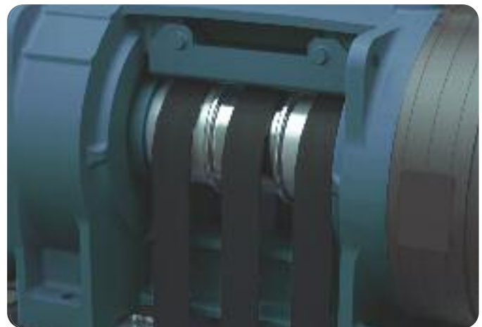
Interaction of Otis' flat belt and the smooth crowned sheave.
