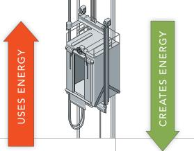
Energy created by your elevator is captured by the ReGen® drive and is put to use—it's fed into your building's electrical grid.
