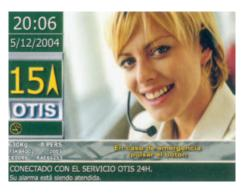
In the new elevator cars, the trunking with the system cables have disappeared, since the whole device leaves the plant fully integrated into the car operating panel, in the place formerly occupied by the elevator display. This saves space and represents a great step forward in the aesthetics of the car.
