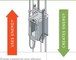
is captured by the ReGen® drive and is put to use—it's fed into your building's electrical grid.
