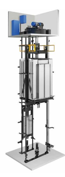
The compact machine-room configuration reduces the footprint of the Gen2 by 16%, so it's no larger than the hoistway footprint, with an additional 9% reduction in machine-room height and a 15% reduction in overhead.
